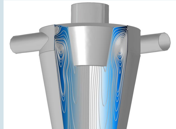
Flow in a hydrocyclone. A typical application where v^2 - f gives superior results over two-equation models such as k - \epsilon or SST.
