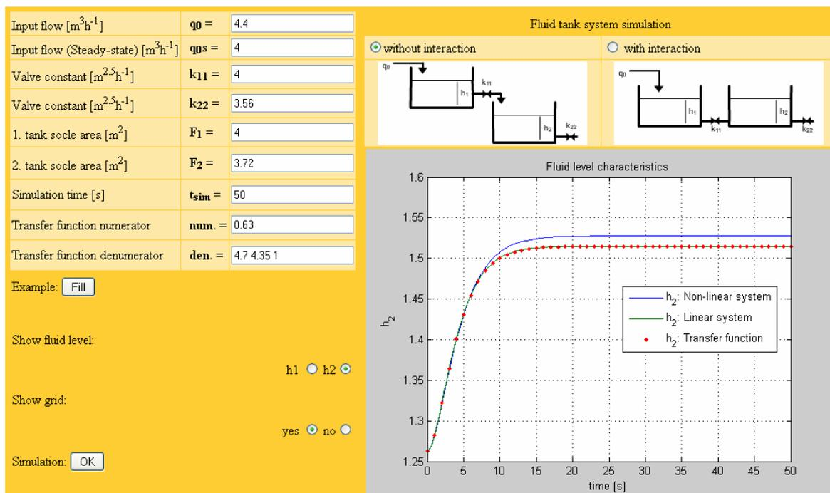
Fig. 3: Storage tank system simulation
