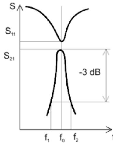
Figure 4: Resonant curve.
