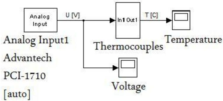
Figure 5: Temperature measurement scheme in Simulink.
