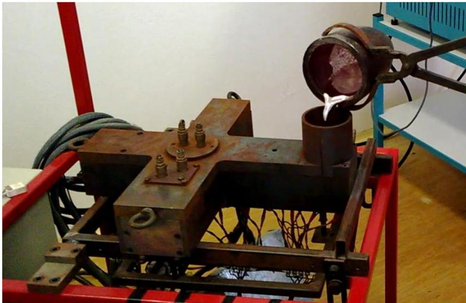
Figure 4: Filling the cavity of foundry mold.
