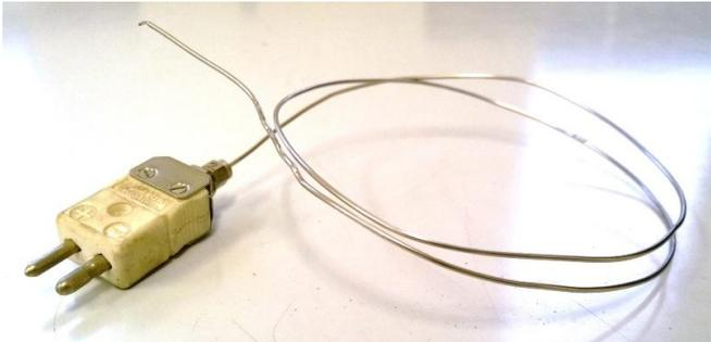
Figure 3: Thermocouple type K, Omega mold [9].
