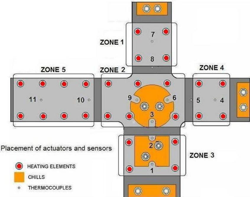
Figure 2: Thermocouples sensing elements, cooling and heating elements located on body of foundry mold [3].
