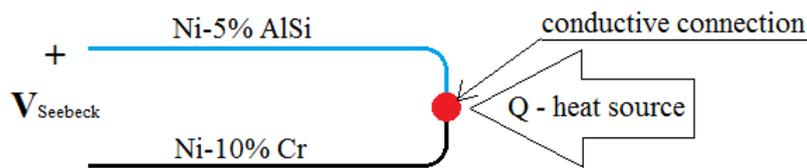
Figure 1: Seebecks voltage generating scheme [1].
