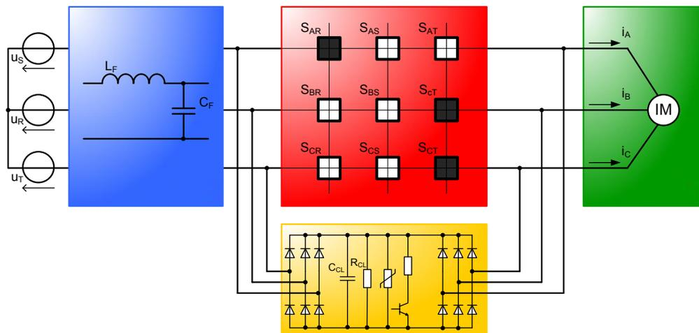
Figure 1: Matrix converter block diagram
