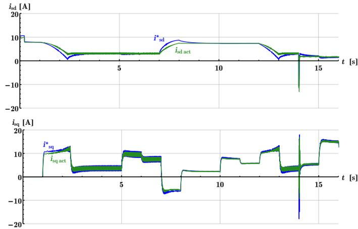
Figure 6: Vector control simulation – reaction to torque steps
