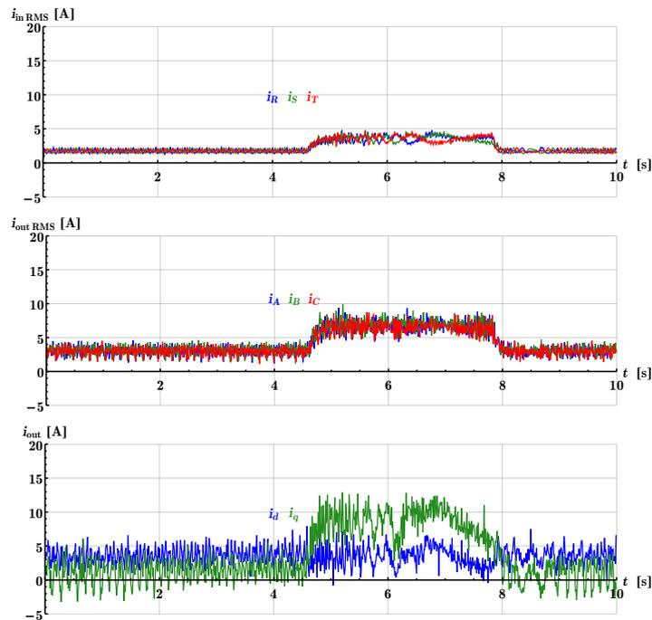
Figure 8: Vector control realization – reaction to torque step
