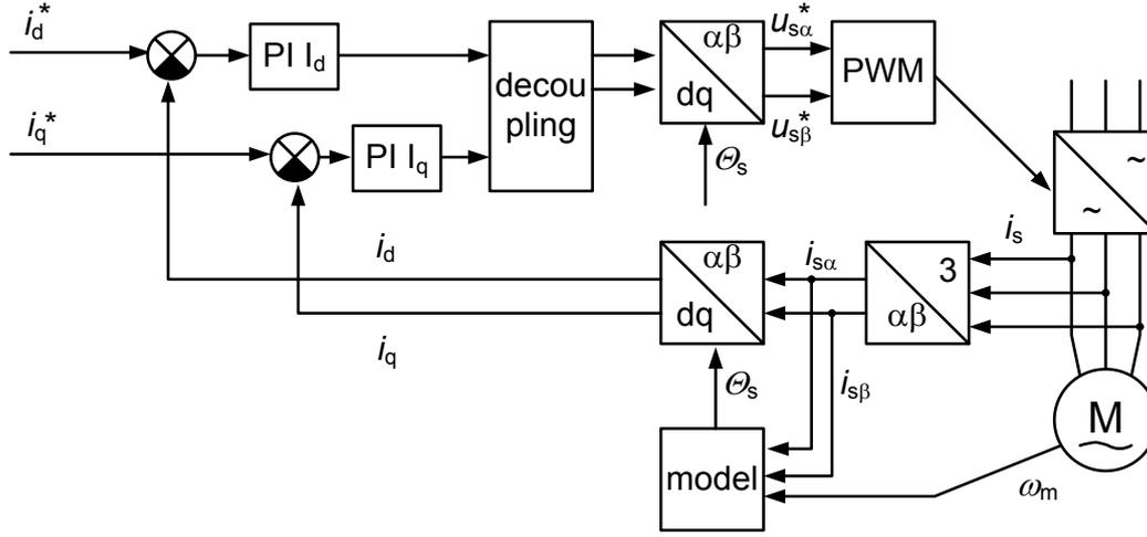
Figure 3: Vector control block diagram
