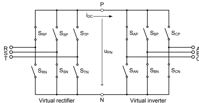
Figure 2: Matrix converter ISVM model
