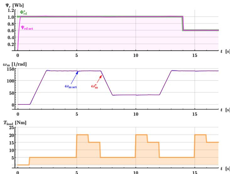
Figure 5: Vector control simulation
