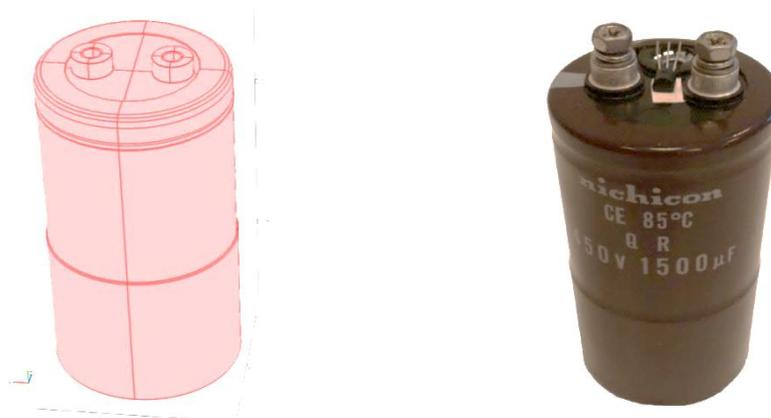
Fig. 7. Left - geometric model of the capacitor, right - examined capacitor with glued temperature sensor
