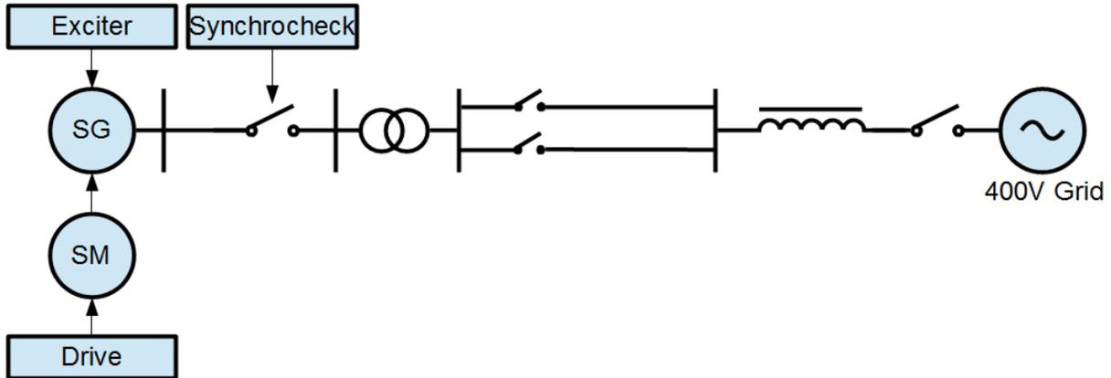
Figure 1: The basic block diagram of the proposed power plant model
