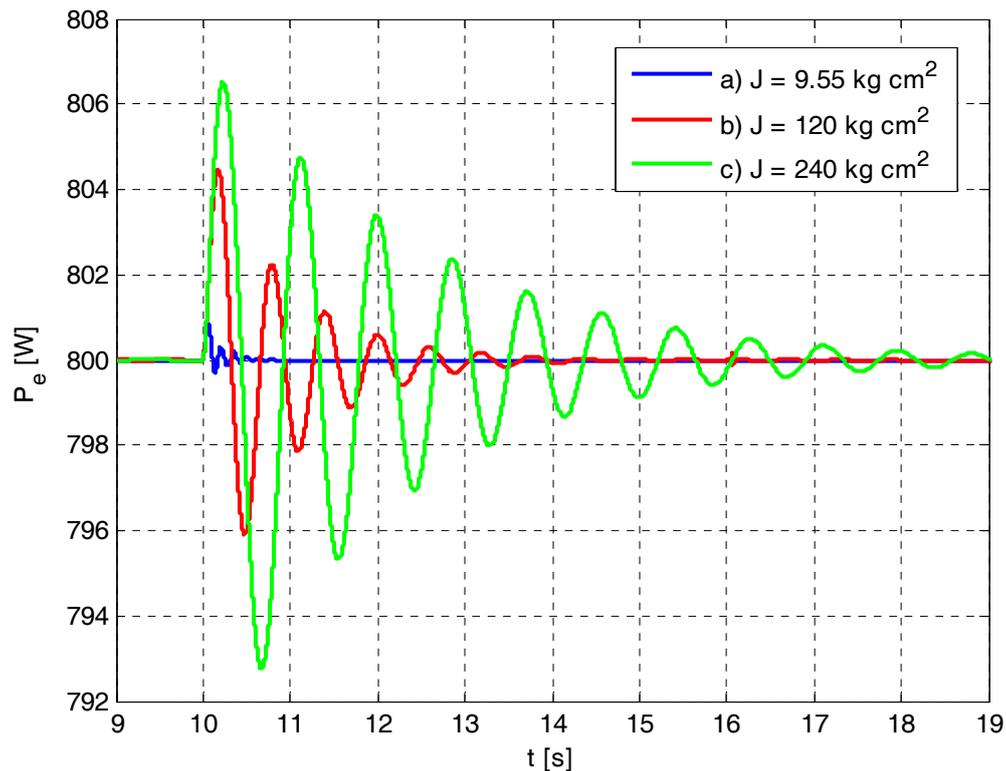
Figure 7: The electric power of synchronous generator response to the step change of excitation voltage
