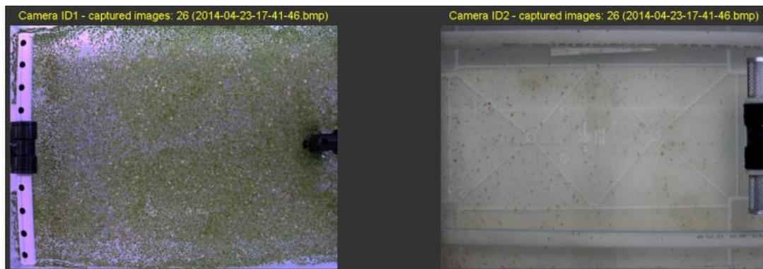
Figure 3: Input images from the colour CCD cameras: Lemna minor (left) and Daphnia magna (right)
