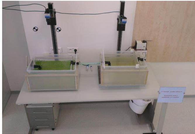
Figure 2: The isolated vessels containing different bio-organisms and a camera subsystem
