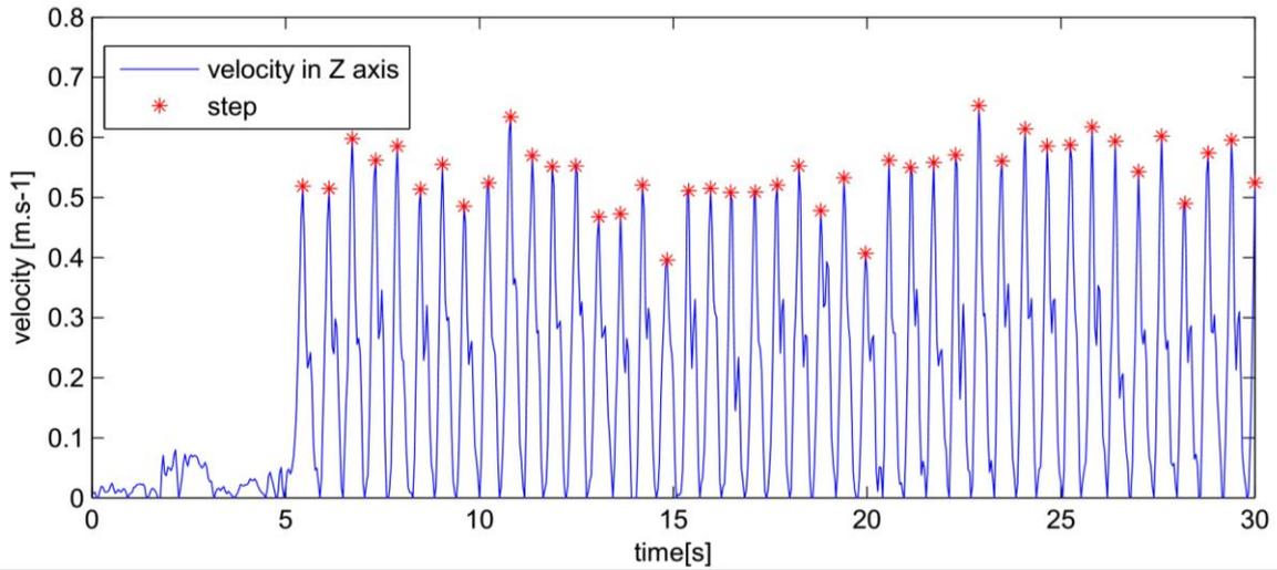
Figure 4. Preview of the step detection from the velocity in direction of the Z axis
