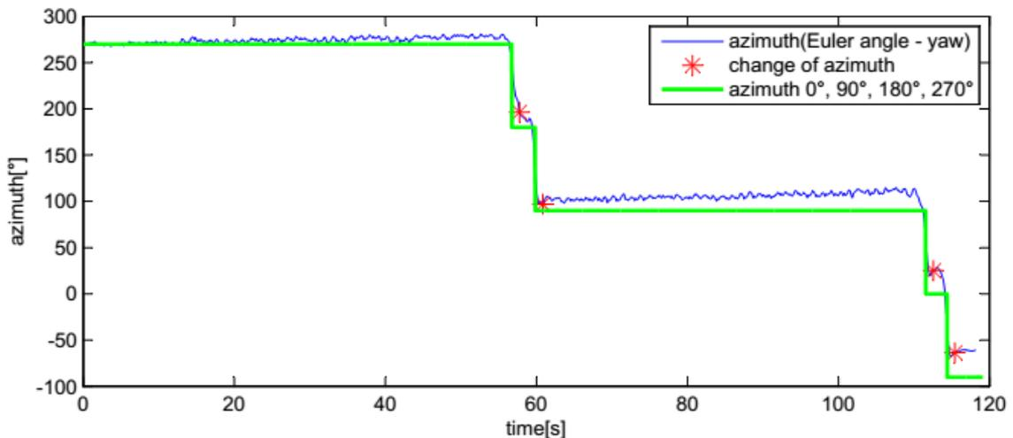
Figure 5. Orientation of pedestrian limited to four basic directions when trajectory is rectangle
