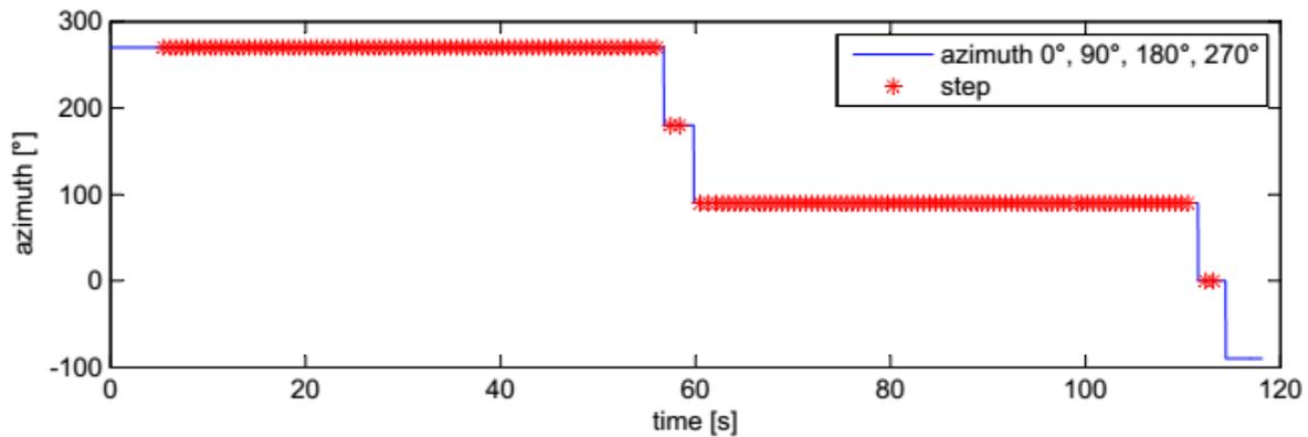
Fig. 6. Steps in the orientation limited to four basic directions
