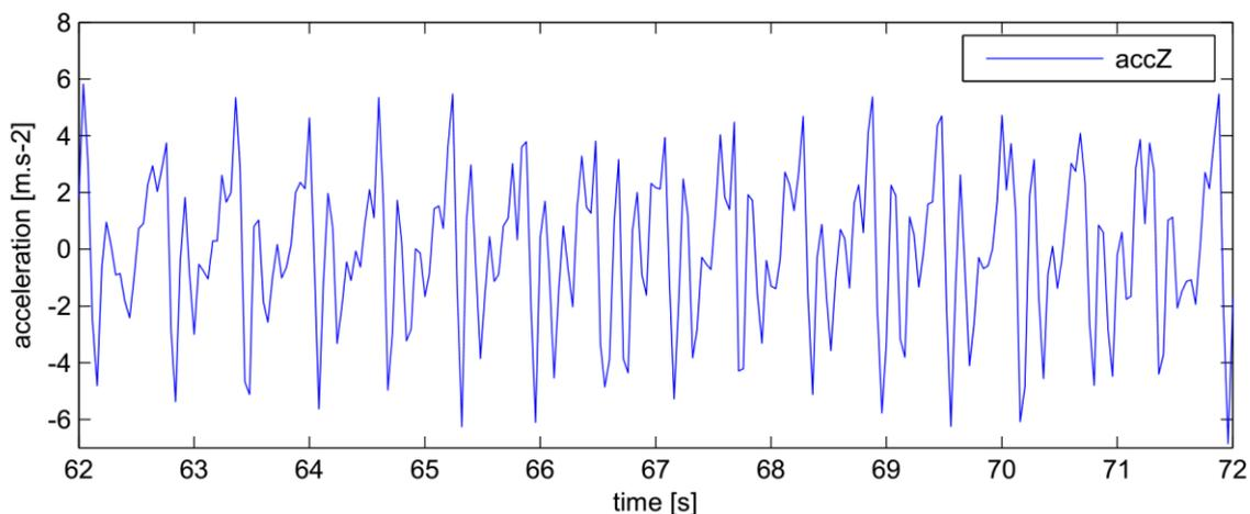
Figure 3. Preview of the calibrated values from the acceleration sensor corresponding to the z axis while walking
