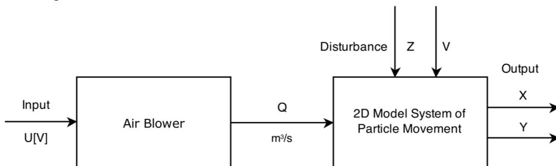
Figure 2: Input-output block scheme of the model system
