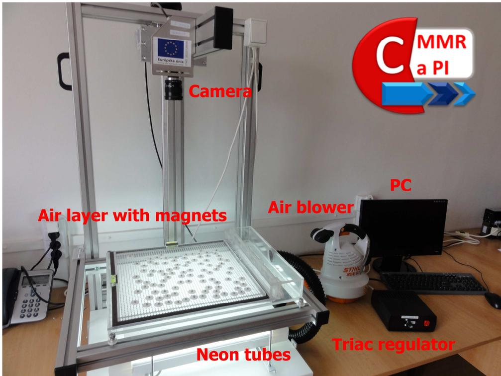
Figure 1: Simulation of particle movement in a two-dimensional system using a mechanical model of small magnets
