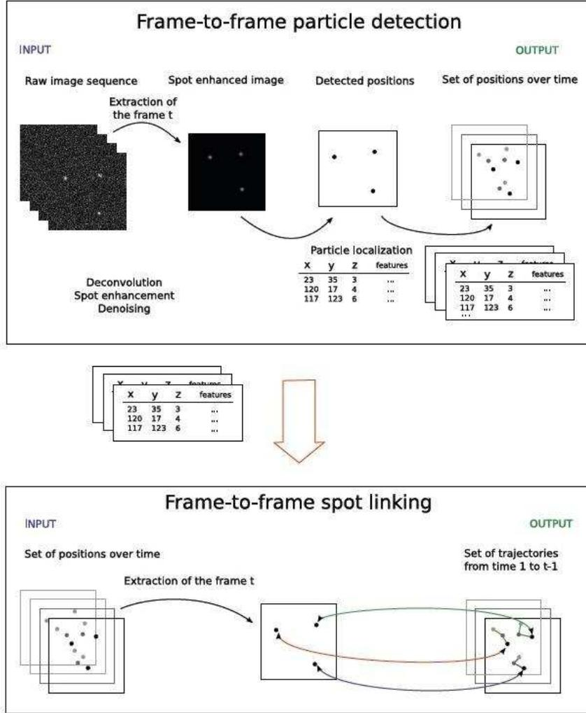
Figure 4: Standard two-step procedure for obtaining trajectories, implemented in *Magtrack* [9]
