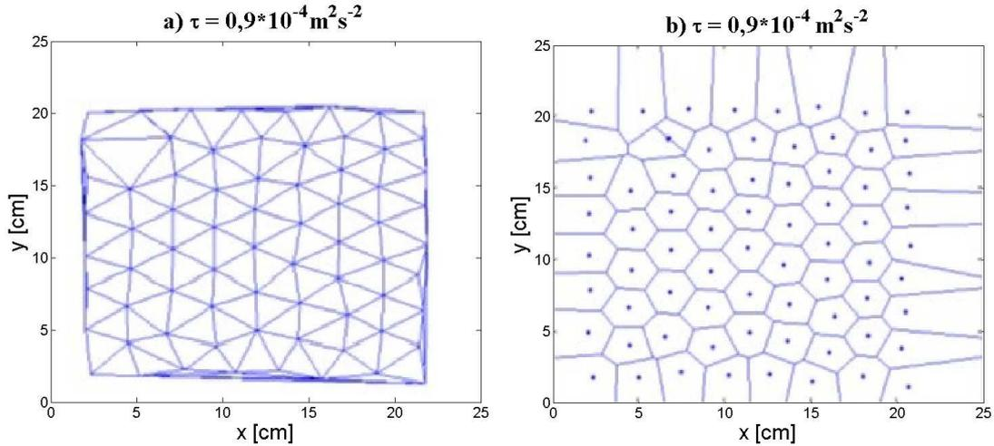
Figure 10: a) Delaunay triangulation b) Voronoi diagram for a low  $\tau$  – crystal phase
