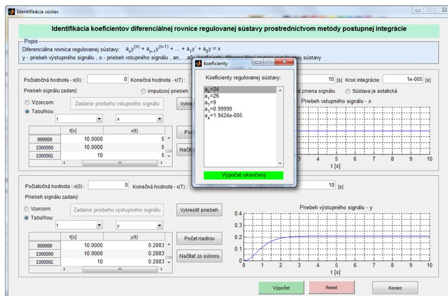
Figure 4: The calculated coefficients of differential equation of the regulated system.
