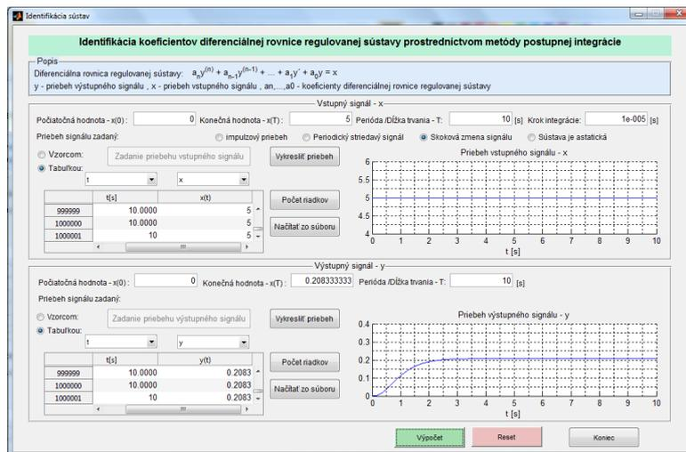
Figure 3: Program for calculating the differential equations using the gradual integration method.
