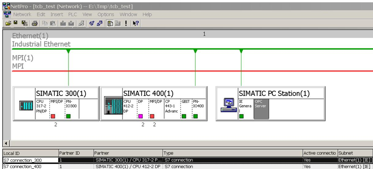
Figure 2: Configuration of connections in NetPro
