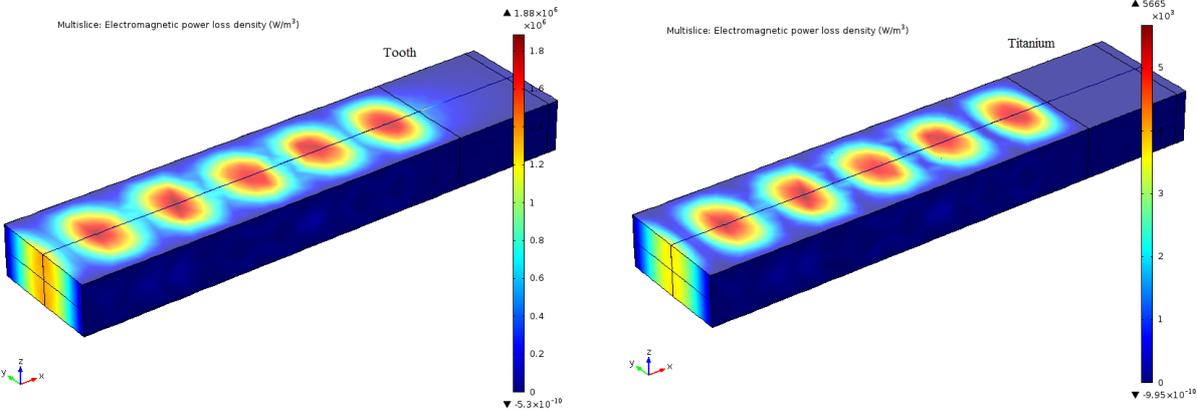
**Fig. 1: Rectangular waveguide WR – 90 filled with air and with dielectric material: tooth (left side) and titanium as replacement (right side) at 12 GHz (electromagnetic power loss density)**
