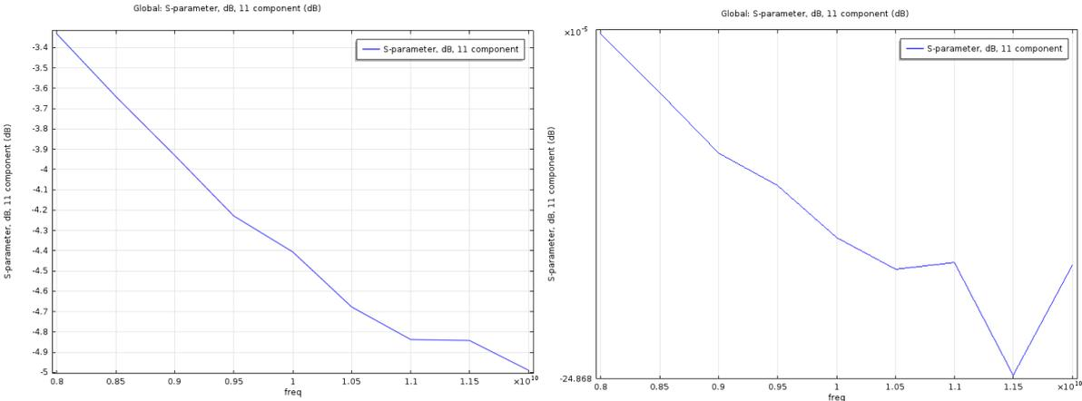
**Fig. 2:  $S_{11}$  parameter: for short-circuited waveguide filled with tooth (left side) and titanium (right side) at 8 - 12 GHz**
