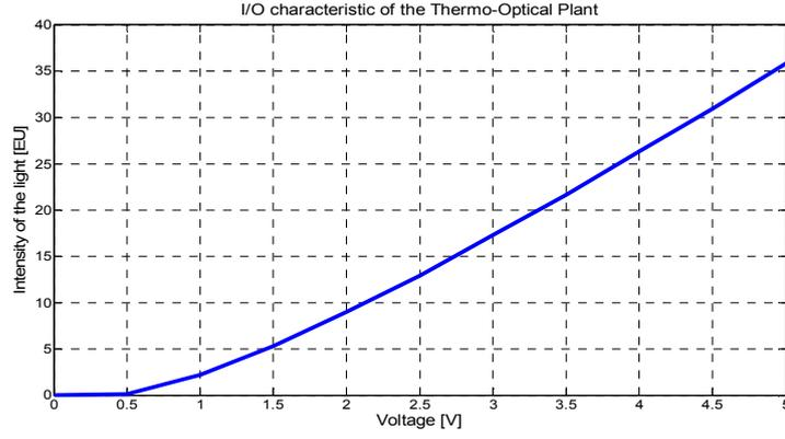
Figure 3: I/O characteristic of the thermo-optical plant
