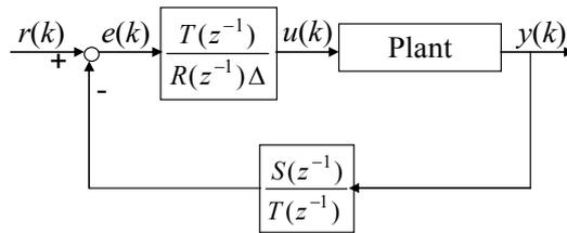
Figure 1: MPC structure
