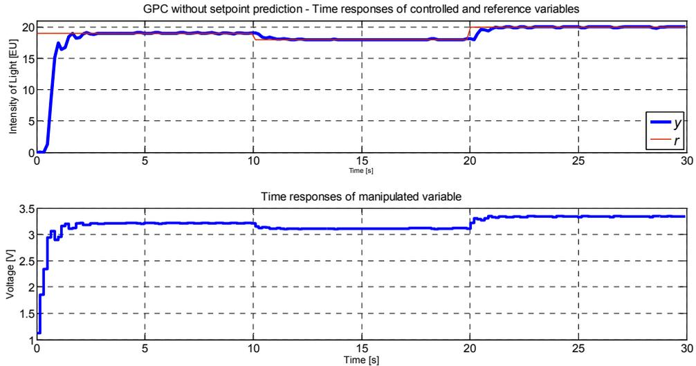
Figure 4: Time responses of the variables under GPC (without setpoint prediction)
