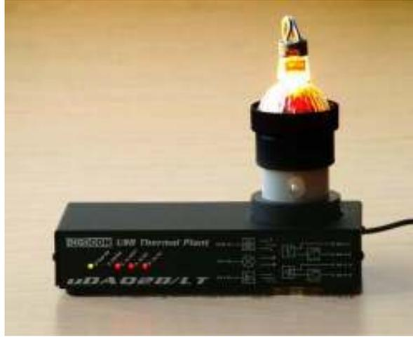
Figure 2: Thermo-optical plant
