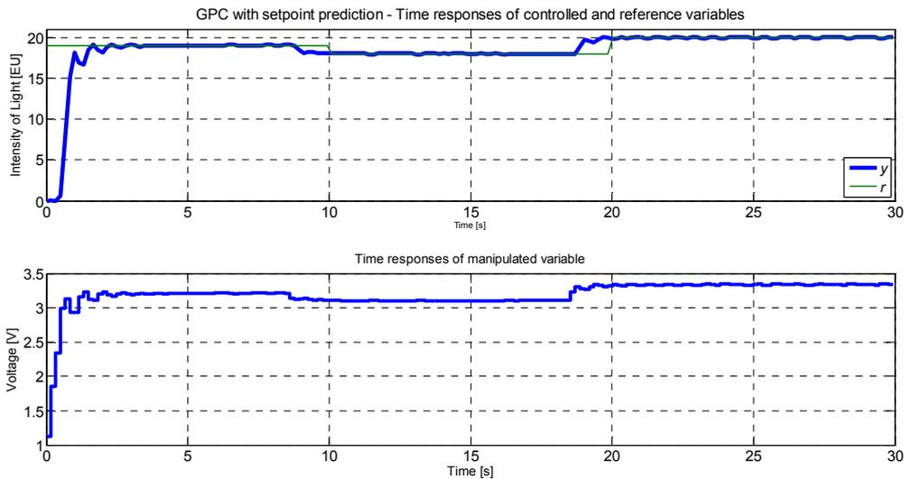
Figure 5: Time responses of the variables under GPC (with setpoint prediction)
