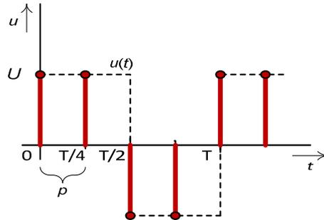
Figure 1: Impulse switching function of single phase voltage inverter system
