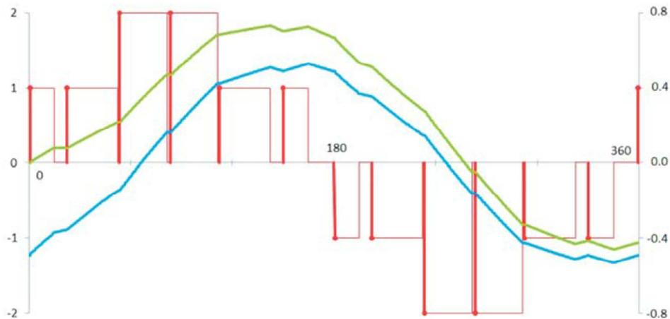
Figure 4: State variable response under sine PWM supply [6]
