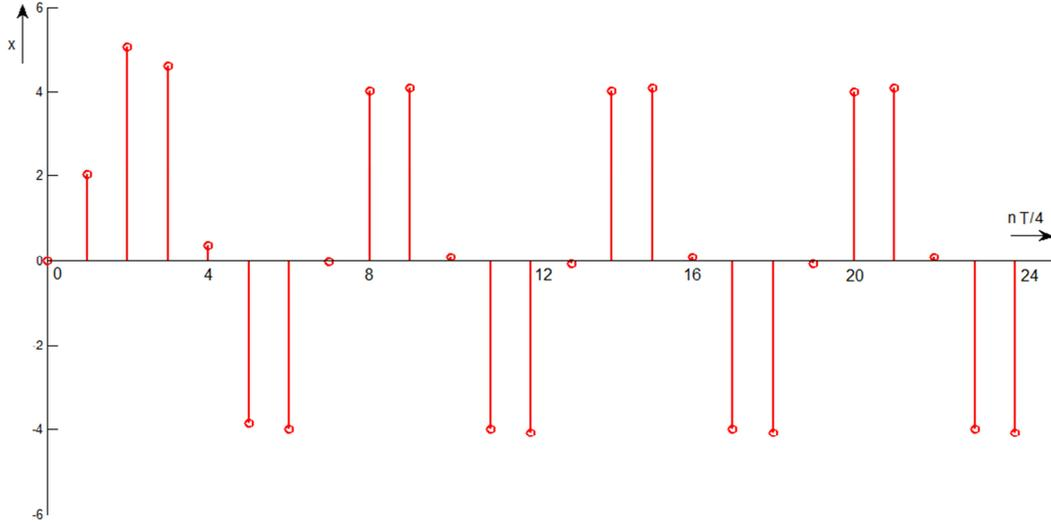
Figure 3: Discrete response sequence of state-variable  $x\left(n\frac{T}{4}\right)$  of single-phase inverter
