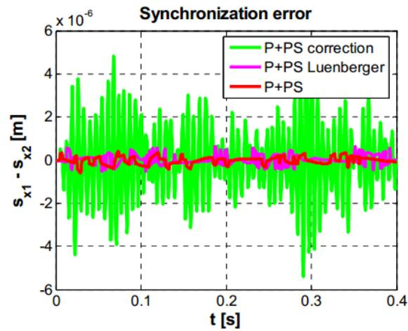
Figure 9: Comparison of the measure of synchronization error control structure of the dual drive gantry stage model
