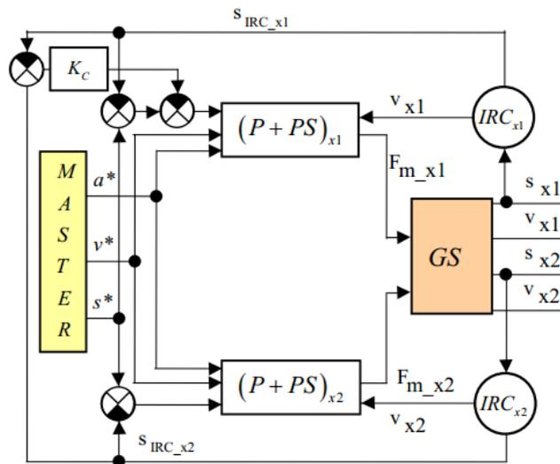
Figure 6: Schematic representation of P+PS cascade control structure with correction
