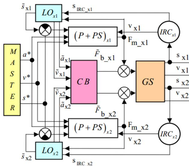
Figure 8: Schematic representation of P+PS cascade control structure with Luenberger observers
