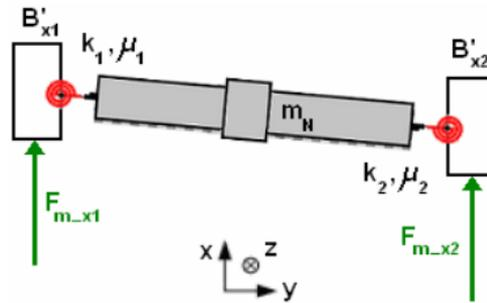
Figure 2: Dual-drive gantry stage model with elastic elements on both sides
