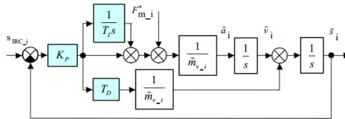
Figure 7: Schematic representation of Luenberger observer
