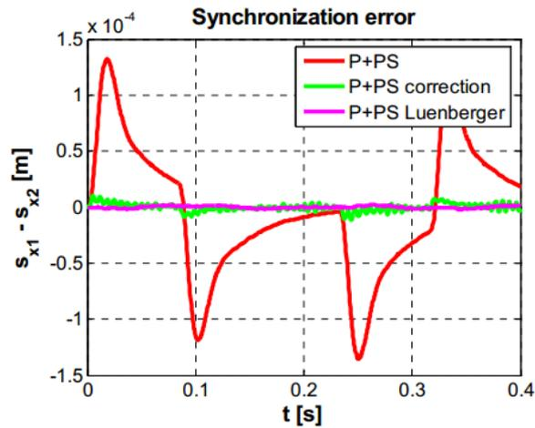
Figure 10: Comparison of the measure of synchronization error control structure of the dual drive gantry stage model
