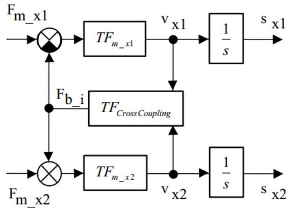
Figure 5: Schematic representation of dual drive gantry stage model
