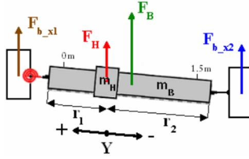
Figure 4: Distribution of the breaking force and initial point of the y-axis of the dual-drive gantry stage model
