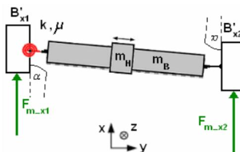
Figure 3: Dual-drive gantry stage model with one elastic element with considering the weight of the head
