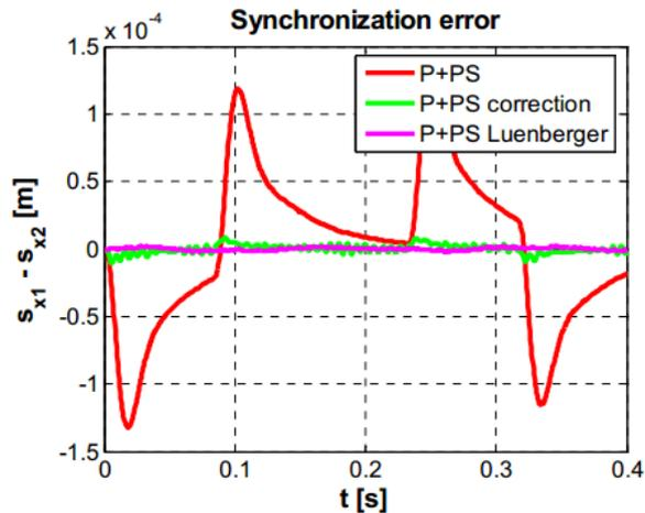
Figure 11: Comparison of the measure of synchronization error control structure of the dual drive gantry stage model
