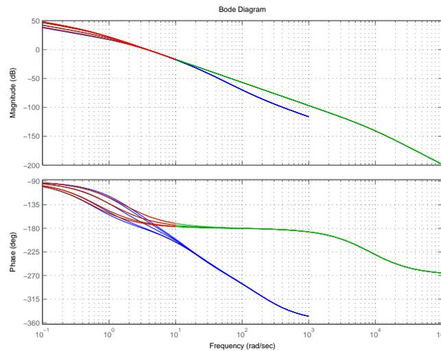
Figure 3: Comparison of the mathematical model and simplified model and real servomechanism
