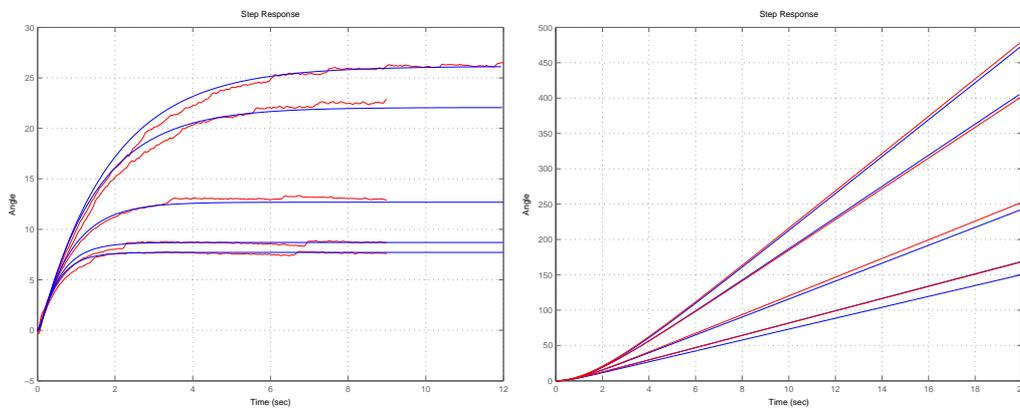
Figure 2: Step and impuls response model and real servomechanism
