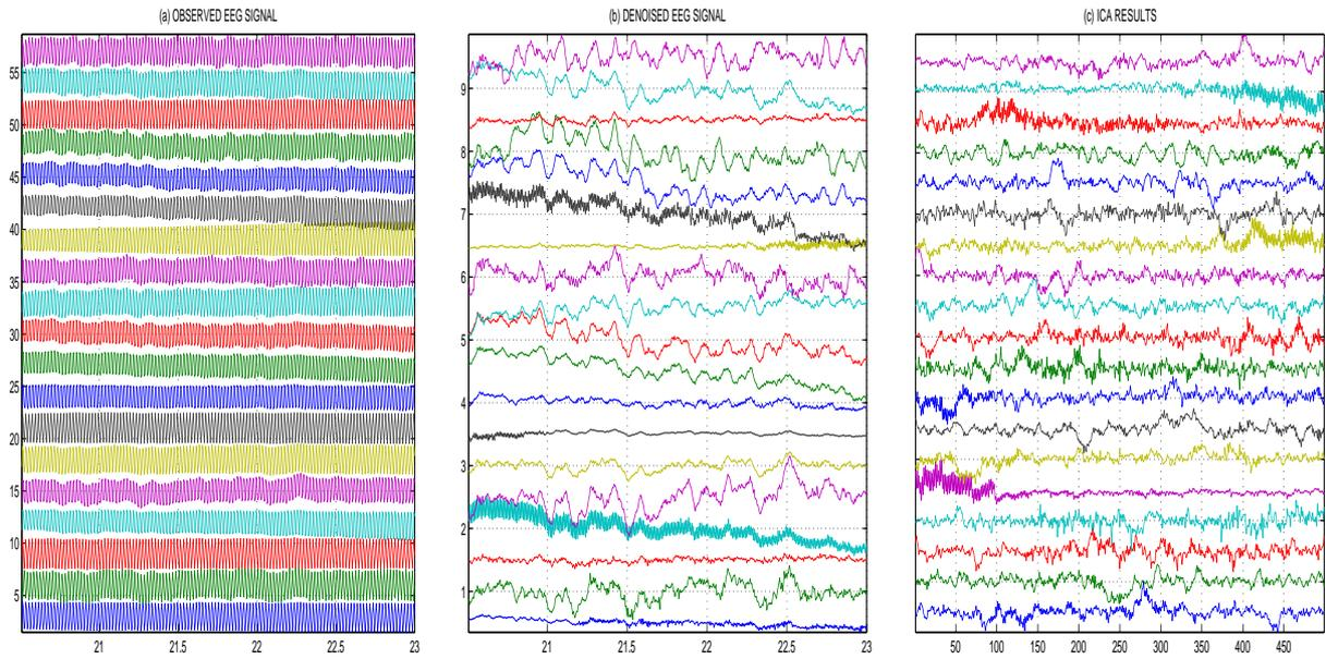
Figure 3: EEG Signals processing presenting (a) original signals sampled at rate of 200Hz, (b) signals obtained after the stop band filtering, and (c) signals (sources) obtained by ICA
