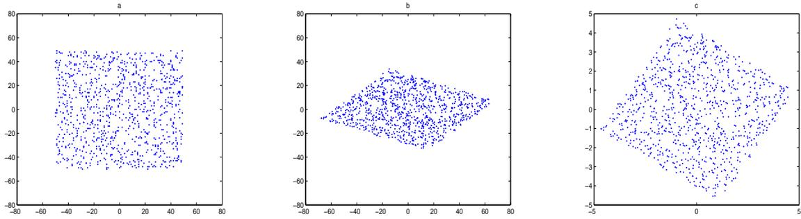
Figure 2: Whitening presenting (a) the joint distribution of the independent components  $s_1$  and  $s_2$  with uniform distributions, (b) the joint distribution of the observed mixtures  $x_1$  and  $x_2$ , and (c) the joint distribution of the whitened mixtures  $z_1$  and  $z_2$
