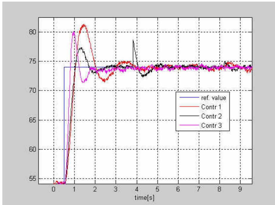
Figure 2: Step responses in the first working point
