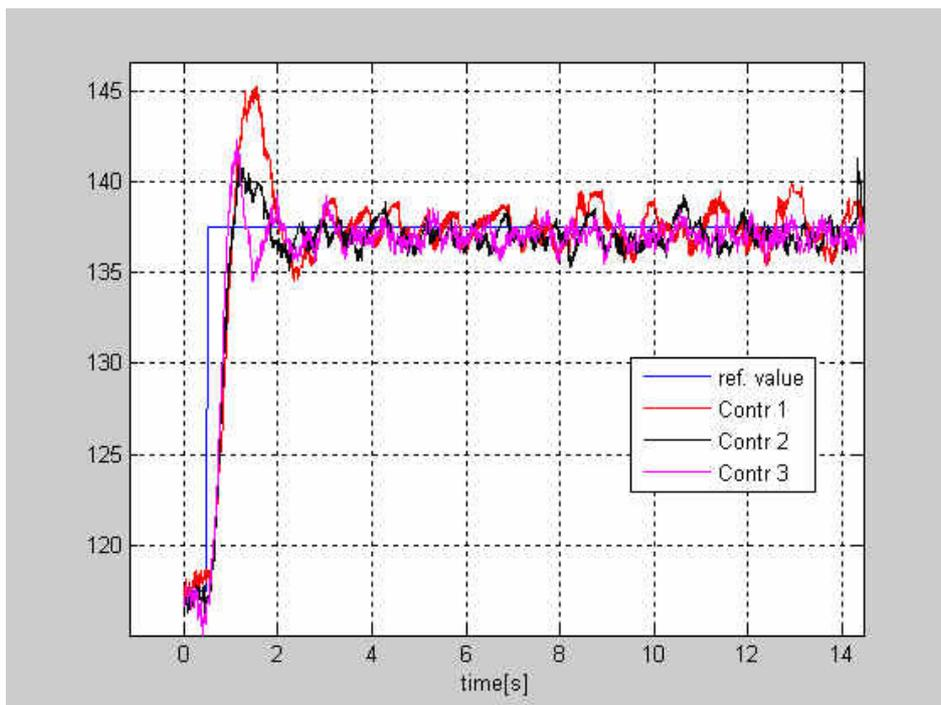
Figure 3: Step responses in the second working point
