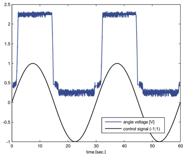
Figure 4. Slow sinus input and response of the system
