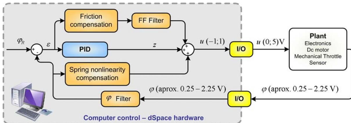
Figure 9. Schema of nonlinear controller
