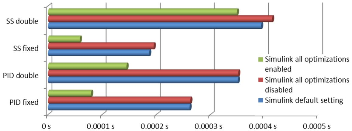
Figure 8: Computing time affected by setting different optimisations for code generation.
