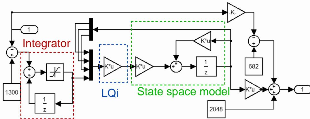
Figure 7: Simulink LQI controller scheme.
