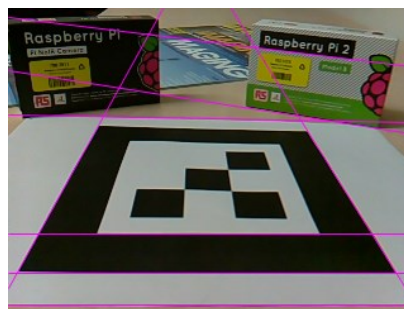
Figure 6: Eight lines related to the eight strongest peaks in the accumulator in the Fig. 5 imprinted into the input image.
