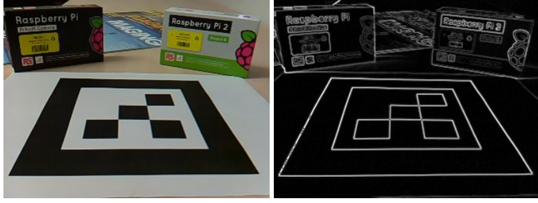
Figure 3: The input RGB image from RPiCam with resolution of 320x240 pixels and the relevant result of the Sobel operator.
